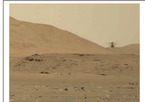
Figure 1: Helicopter flying at an altitude of 5 m above the ground on flight #4 which covered 271 m at 3.5 m/s.
