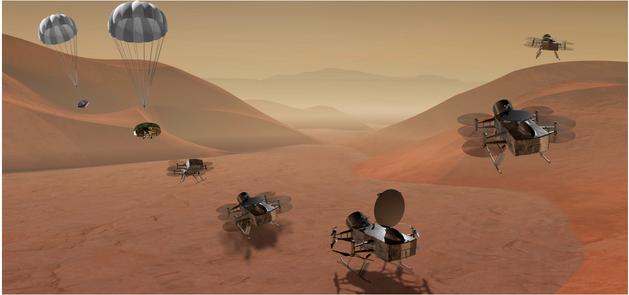
Figure 1. Dragonfly mission concept. After delivery from space in an aeroshell and parachute descent, the vehicle lands under rotor power and deploys a high-gain antenna for DTE communication. Powered by a radioisotope power supply that provides heat and trickle-charges a large battery, the vehicle can operate nearly indefinitely as a conventional lander but can also make periodic brief battery-powered rotor flights to new locations.
