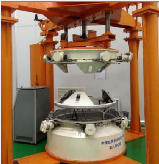
left - Figure 1: The original prototype of docking mechanism and test equipment
