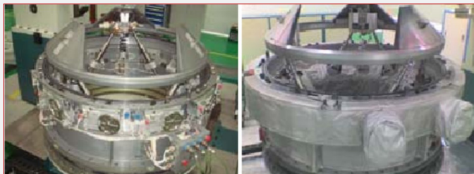
Figure 9: Left is the second set of product docking capability pieces (2008), Right is the third set of product qualification pieces (2009)
