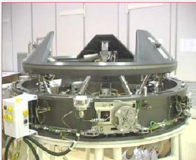
left - Figure 2: The research prototype of docking mechanism (2003.12)
