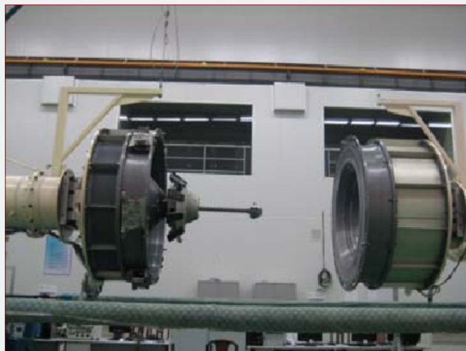
Figure 16: China's Probe-and-Cone docking mechanism
