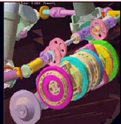
top - Figure 3: The digital prototype of docking mechanism (docking dynamics simulation model) (2004)
