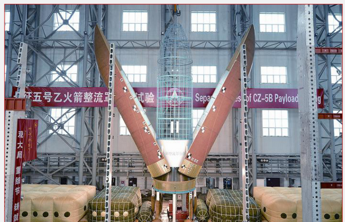
CZ-5's second fairing separation test in June. (credit: Chinese internet)
