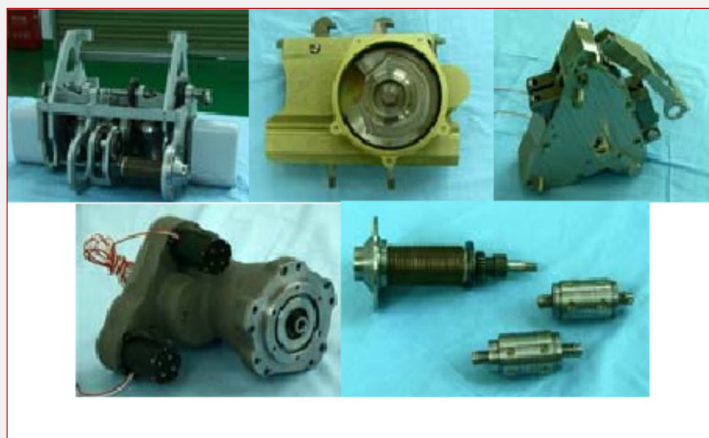
left - Figure 2: The research prototype of docking mechanism (2003.12)
