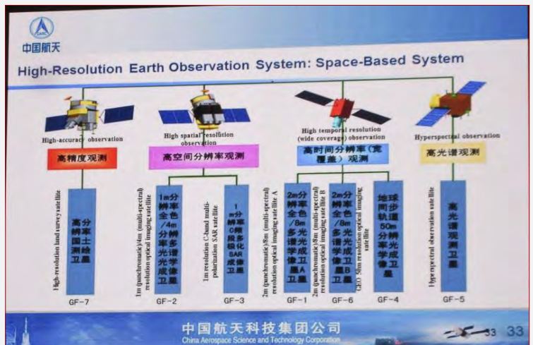
Plan of China's civil high resolution imaging satellites - the Gaofeng (GF) programme. (credit: CASC/Go Taikonauts!)
