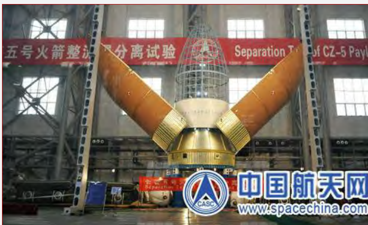
Long March 5 fairing separation test (credit: spacechina.com)
