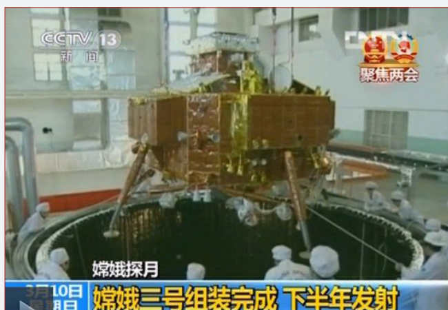
Chang'e 3 undergoing thermal vacuum testing (credit: CCTV)
