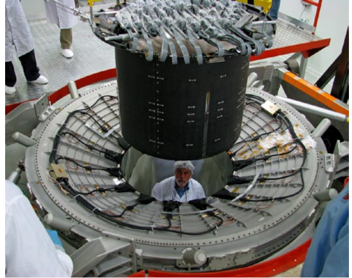
The magnet of AMS-02 during assembly at CERN. (photo: CERN)
