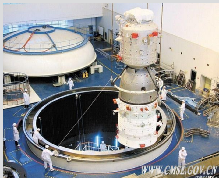
Shenzhou 8 during thermal vacuum test
