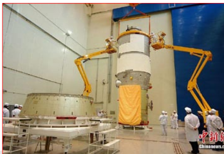
Tiangong 1 during final test and launch preparation. Please note that cover on the TDRS antenna and the alleged telescopes were removed. (Photo: Chinanews.com)
