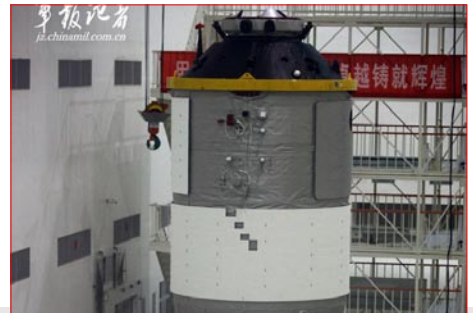
Tiangong 1 during final test and launch preparation. The APAS docking mechanism is seen at the top of the spacecraft and the TDRS antenna in red cloth cover is also seen at its lower section (only in iPad version). (Photo: Chinamil.com)
