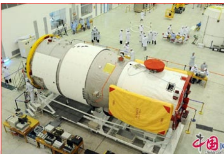
Tiangong 1 during final test and launch preparation. Here the TDRS antenna in red cloth cover is visible to the right. (Photo: China.com)
