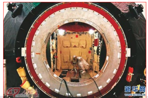
Tiangong 1 interior. Note that a protective plate in this photo covered the docking mechanism. (Photo: Xinhua)
