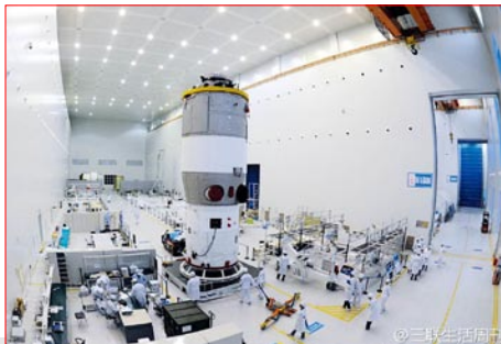
Tiangong 1 during final test and launch preparation. Two telescope-like cylinders are clearly seen at the side of the TG-1's intersecting segment. (Photo: weibo.com/lifeweek)
