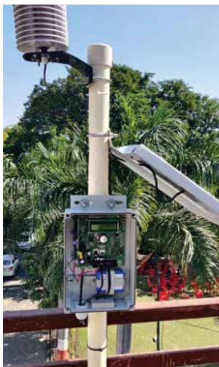
Low-cost air quality sensors were installed at 19 sites in the city of Indore and recorded varied sources of air pollution. Credit: Neeraj Mishra, John Snow India
