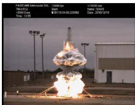
Releasing water into the mesosphere with an explosion (a ground test of which can be seen above) was a key step in forming an artificial noctilucent cloud. Credit: NASA's Wallops Flight Facility
