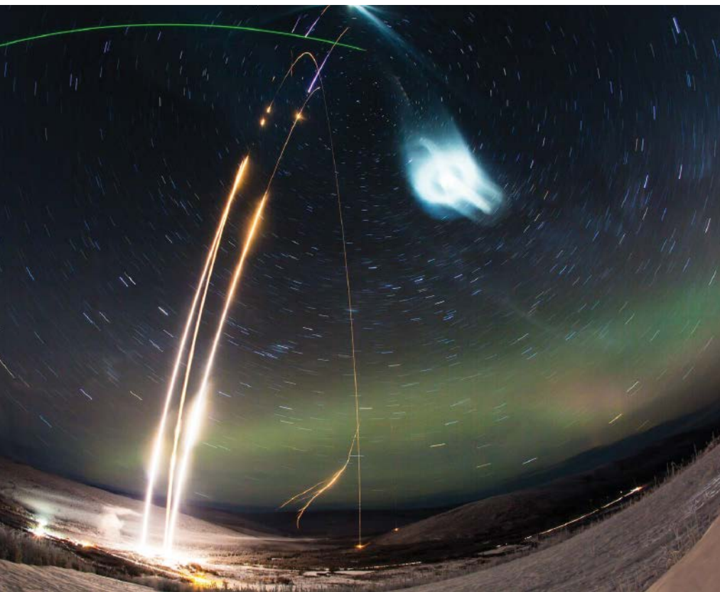
The Super Soaker experiment launched three rockets: One carried a canister of water, and two tracked wind movement (orange trails). A lidar beam (green trail) was used to study the resulting noctilucent cloud (bright white). Credit: NASA's Wallops Flight Facility/Poker Flat Research Range/Zayn Roohi
