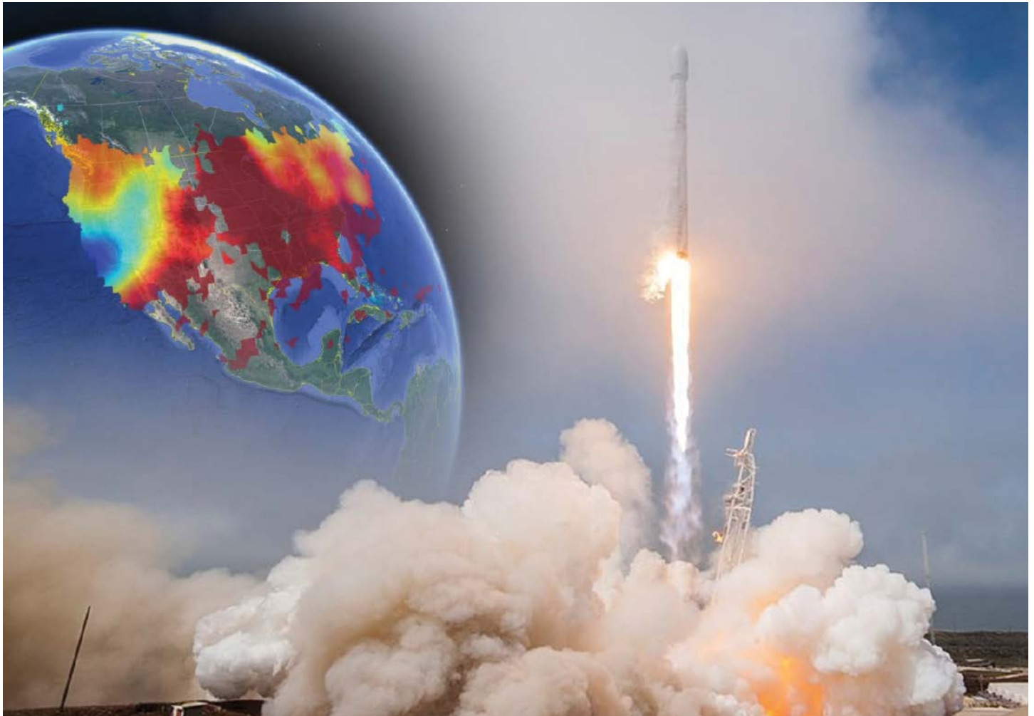
The August 2017 launch of Taiwan's Formosat-5 satellite atop a SpaceX Falcon 9 rocket and the resulting plasma hole over the western United States. Credit: SpaceX
