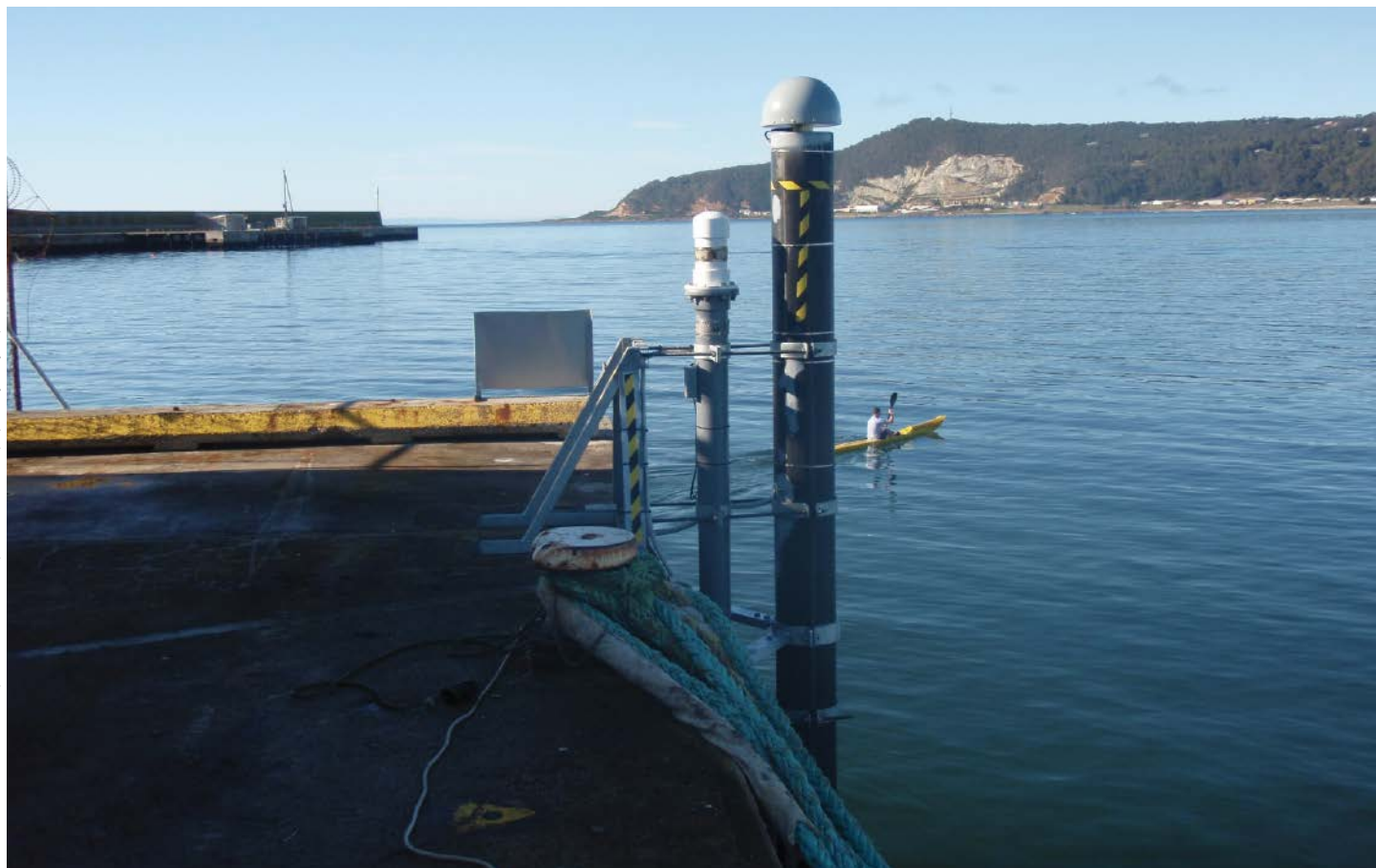
An acoustic tide gauge monitors the harbor at Burnie on the northern coast of Tasmania, Australia. To its right, a special pillar has a GNSS receiver on top.
