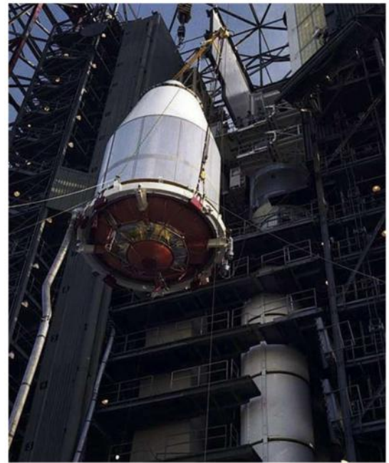
△ Voyager 2, encased in its launch capsule, is winched into position atop the Titan III-E-Centaur rocket
