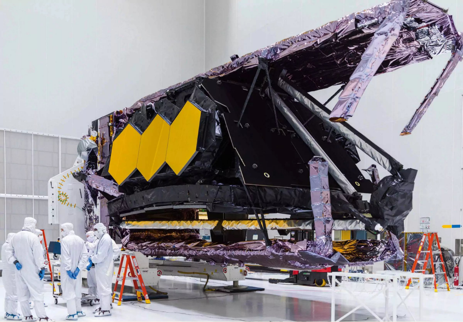
ABOVE LEFT The James Webb Space Telescope's primary mirror measures 6.5m in diameter when fully deployed
