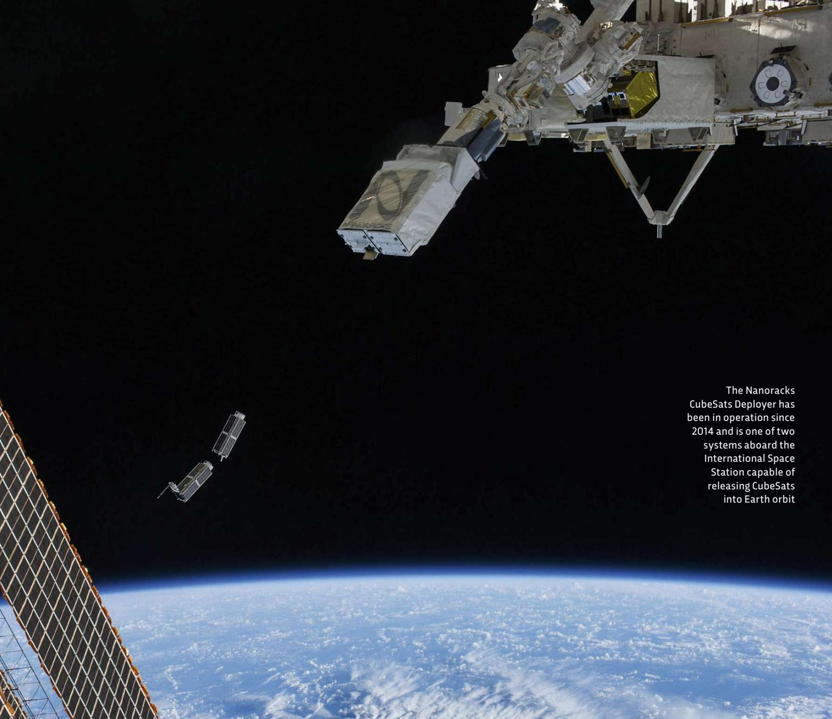
The Nanoracks CubeSats Deployer has been in operation since 2014 and is one of two systems aboard the International Space Station capable of releasing CubeSats into Earth orbit
