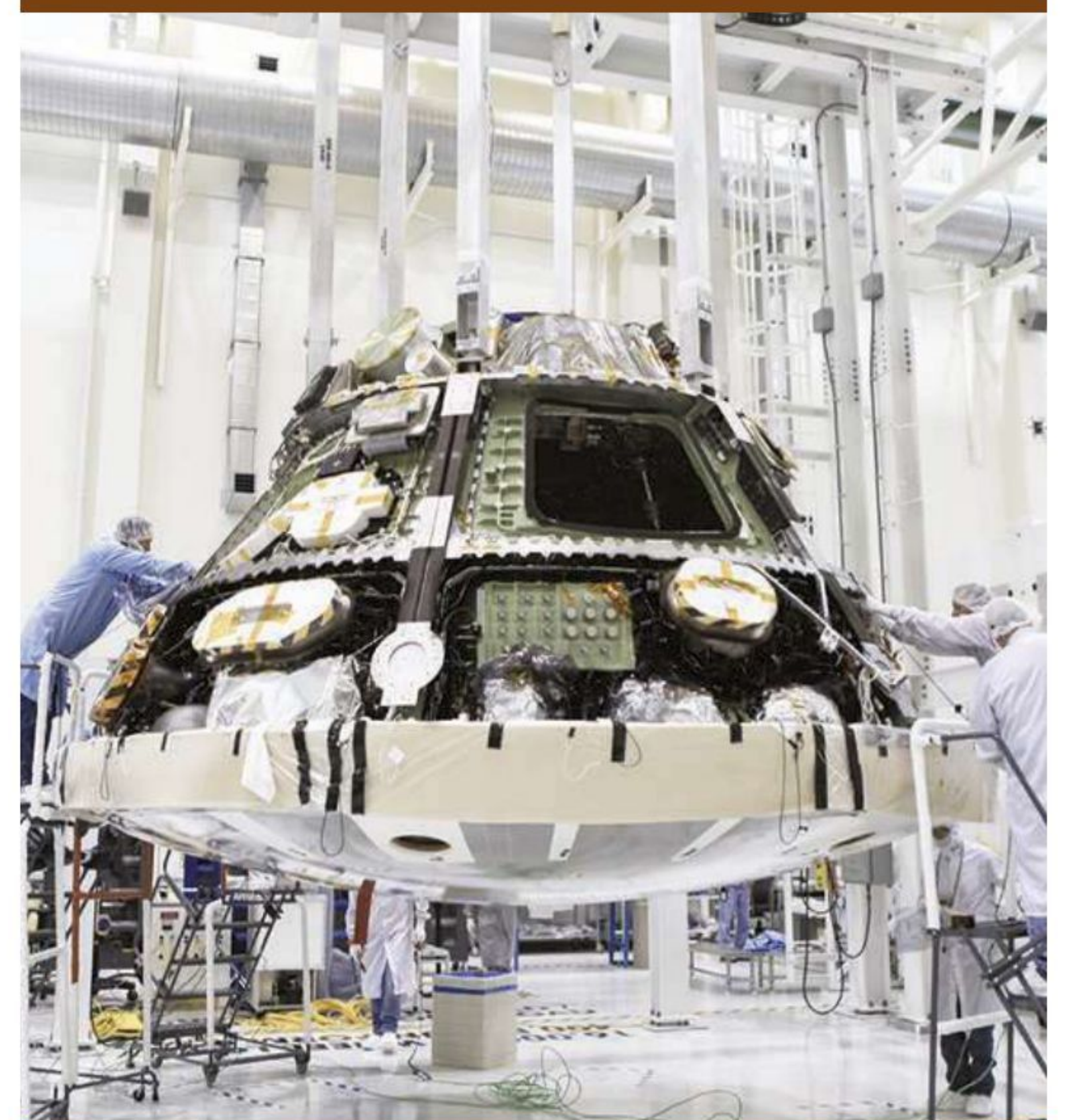
Orion undergoing final assembly at the Kennedy Space Center. Technicians ensured that no foreign objects contaminated the spacecraft
