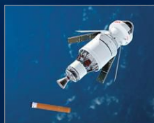
3 Core stage main-engine cutoff and separation. ROEN KELLY AFTER ESA AND NASA
