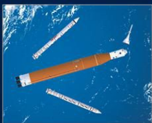
2 Solid rocket boosters, fairings, and launch abort system jettisoned. ROEN KELLY AFTER NASA
