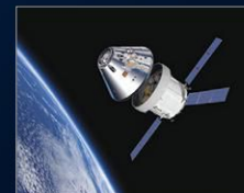
12 Crew Module separates from Service Module. ROEN KELLY AFTER NASA
