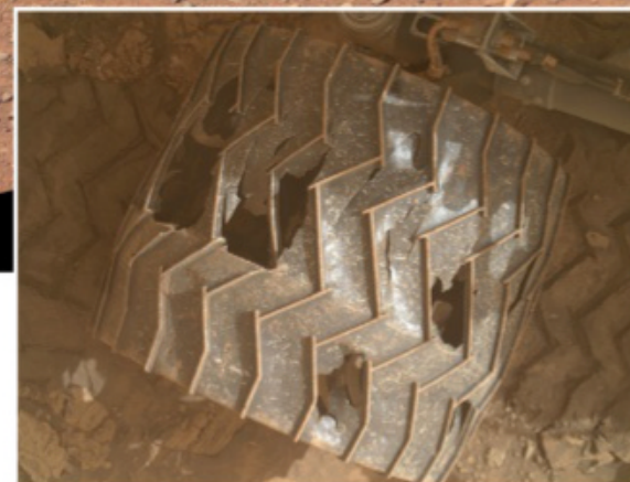
RIGHT: Over time, the tough martian terrain has damaged Curiosity's wheels. The result of such wear and tear is visible in this image, snapped by the MAHLI instrument Jan. 27, 2022. NASA/JPL-CALTECH/MSSS
