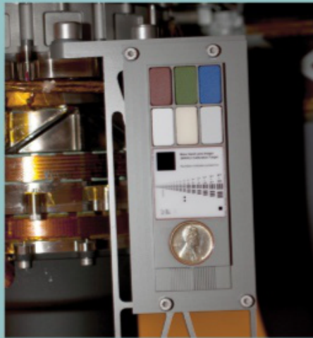
MAHLI’s calibration target is located near one of the robotic arm’s shoulder joints. The target includes color chips, a bar graphic, and a 1909 Lincoln penny. NASA/JPL-CALTECH
