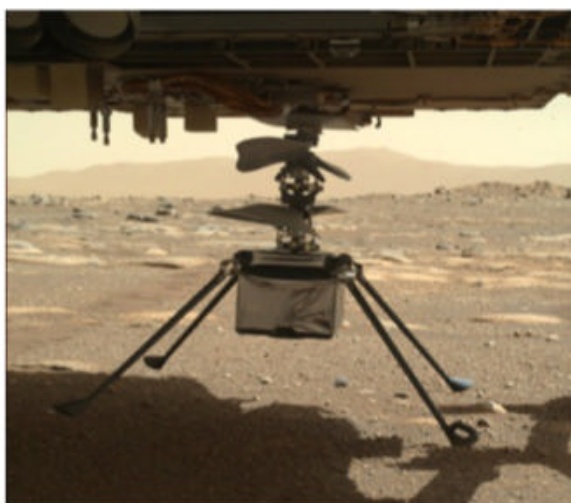
DELIVERY DROP-OFF. Ingenuity has its legs deployed in this photo, ready to drop from the belly of Perseverance, where it stowed away during its journey to Mars. NASA/JPL-CALTECH/MSSS
