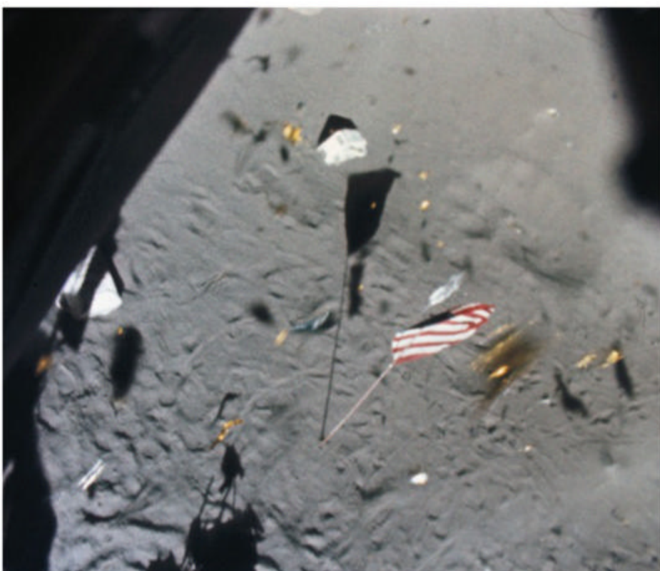
ABOVE: As Antares lifts off, its ascent engine blasts pieces of gold foil off the descent stage and leaves the U.S. flag swinging on its pole.
