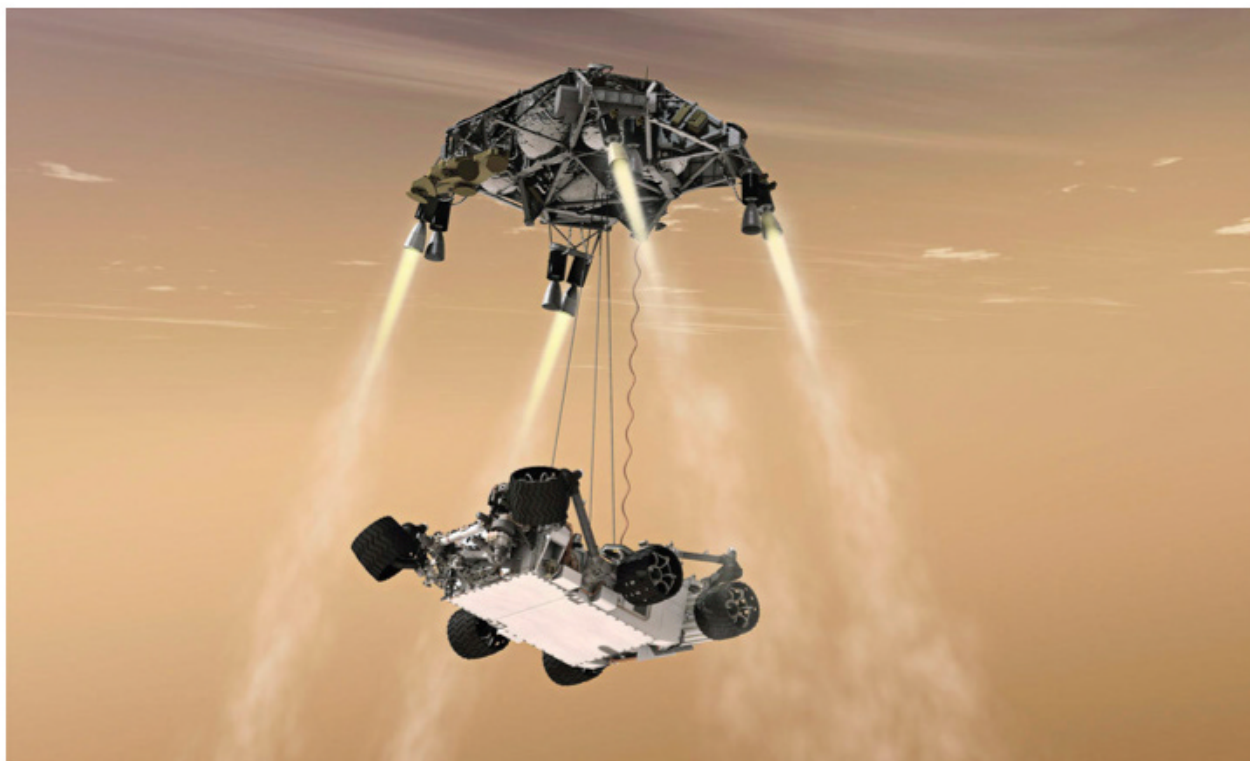
Like Curiosity (shown in this artist's concept), Perseverance will be gently lowered to the ground using a sky crane maneuver. The descent stage will fire retrorockets to slow down before unspooling about 25 feet (7.5 m) of ropes and an "umbilical cord" attached to the rover until Perseverance softly touches down. NASA/JPL-CALTECH
