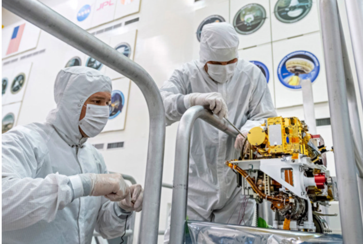
Engineers carefully install SuperCam on Perseverance last June in the Spacecraft Assembly Facility at the Jet Propulsion Laboratory in Pasadena, California. NASA/JPL-CALTECH
