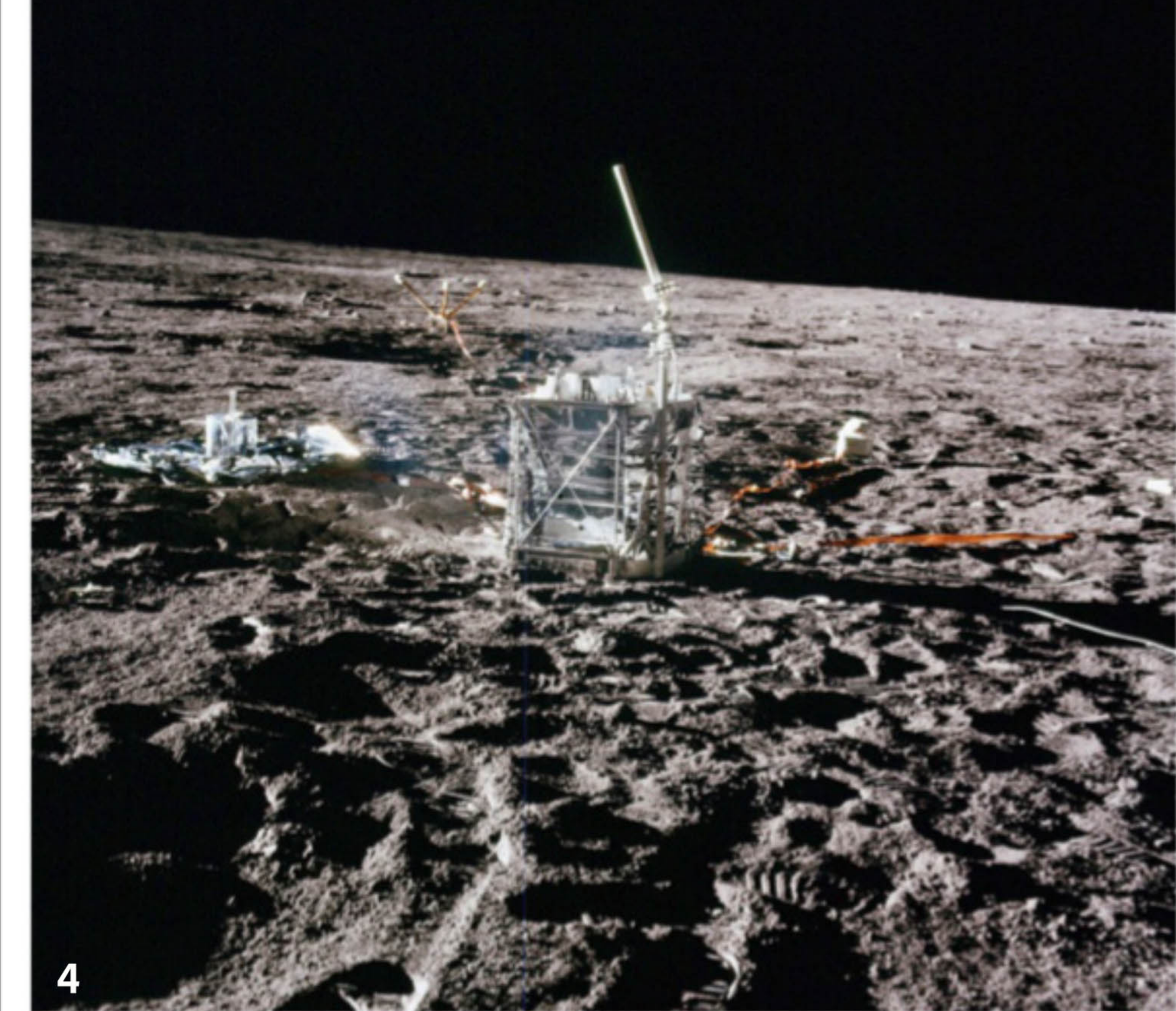
3. Bean lugs the ALSEP suite of instruments away from the LM. The astronauts would deploy the package 410 feet (125 m) northwest of Intrepid. 4. The Central Station, which supplies power and communications between ALSEP and Earth, stands at the heart of the instrument package. The Solar Wind Spectrometer appears to the station's right, the Passive Seismic Experiment to the station's left, and the Lunar Surface Magnetometer in the background.
