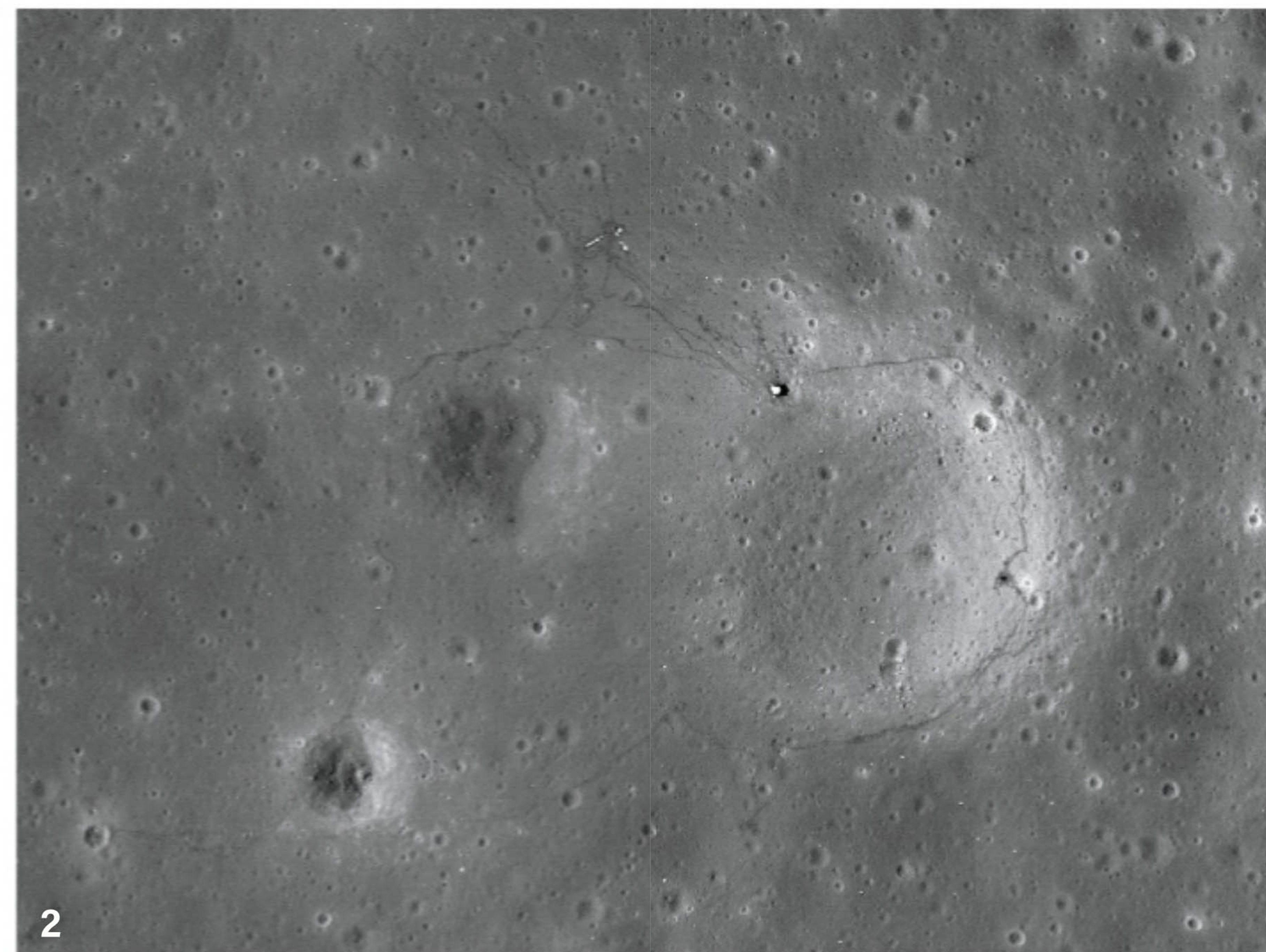
2. The camera on NASA's Lunar Reconnaissance Orbiter captured this view of the Apollo 12 landing site in 2011. The lunar module stands out as the bright object on the edge of Surveyor Crater, while the ALSEP shows up clearly to its upper left. The dark streaks reveal the disturbed soil where the astronauts walked. NASA/GSFC/ASU
