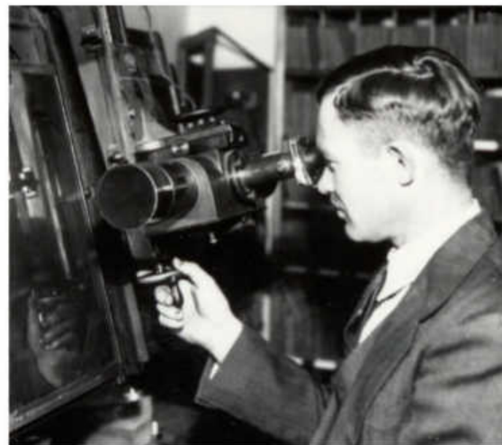
Clyde Tombaugh, Pluto's discoverer, peers through the "blink comparator" he used to identify tiny, dim Pluto on the photographic plates.
