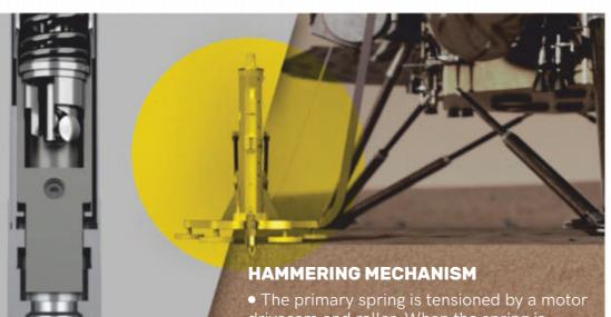
The primary spring is tensioned by a motor drivecam and roller. When the spring is released, it drives the hammer forward.
