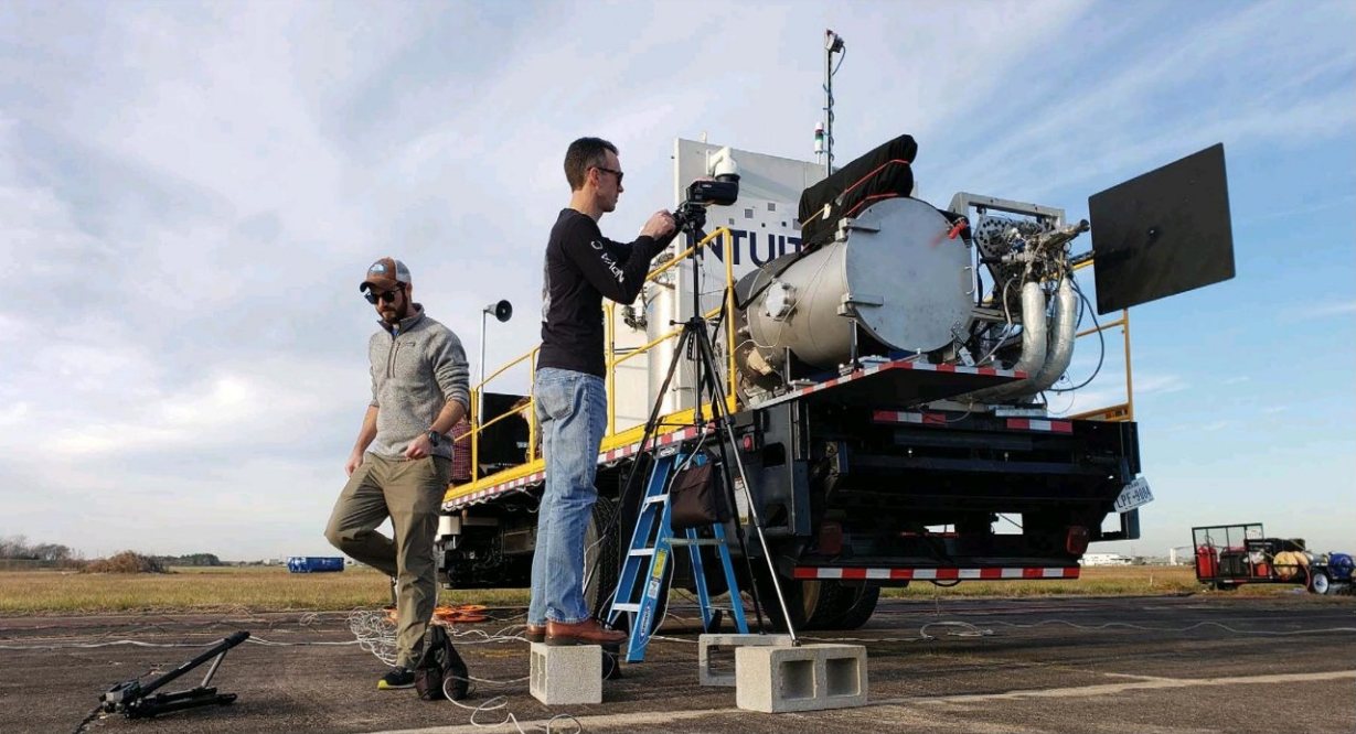
↑ Using the firm's converted flatbed-truck mobile test stand on a Houston runway, IM engine designer Rob Morehead (right) makes final adjustments prior to a hot-fire test of an engine for the Nova-C lander.
