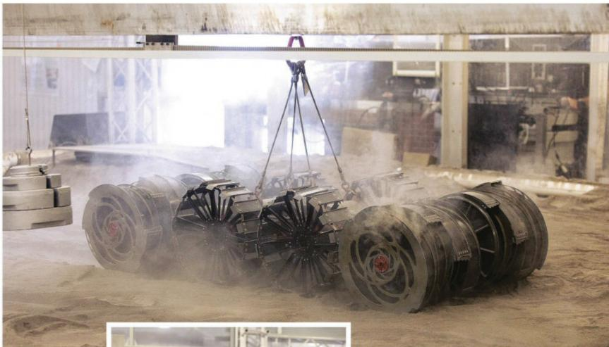
Initially, NASA plans to use a drill to locate ice deposits on the moon, but digging a trench might prove to be more effective. A digging robot named RASSOR (top, undergoing tests at NASA's Kennedy Space Center in Florida on June 5, 2019) will excavate regolith with rotating bucket drums fitted with toothy digging scoops (bottom), each capable of holding 60 kilograms.
