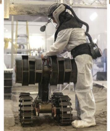
through a patent-pending process called radiant gas dynamic (RGD) mining, which uses a combination of radio-frequency heaters, microwave, and infrared radiation to heat permafrost and other types of ice deposits.
