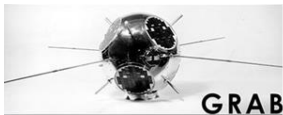
Figure 11–5: GRAB satellite. The solar panels for energy and the antennas along its spherical shape were really characteristic of GRAB. Source NRO.
