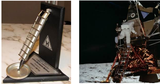
Figure 6–16: Apollo Lunar Module landing gear developed by Héroux.
