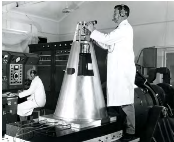
Figure 15–6: WRESAT being readied for vibration testing on a shaker-table constructed in-house by the Weapons Research Establishment. Credit: Defence Science and Technology Group.
